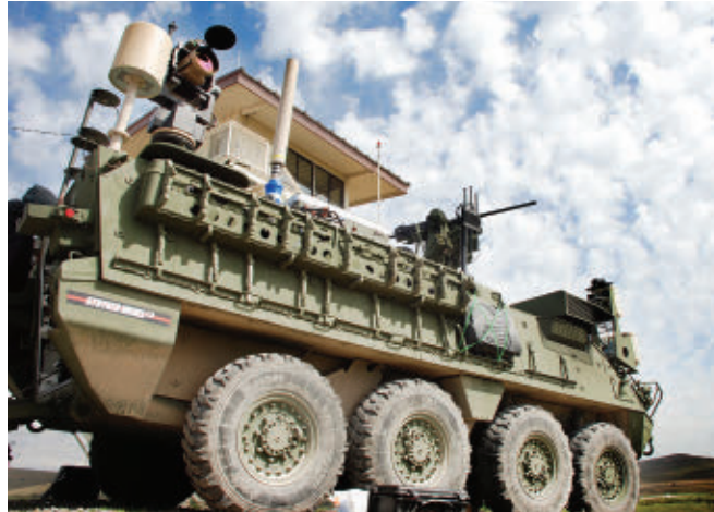
This Mobile High-Energy Laser-equipped Stryker was evaluated last during the 2017 Maneuver Fires Integrated Experiment at Fort Sill, Okla.
