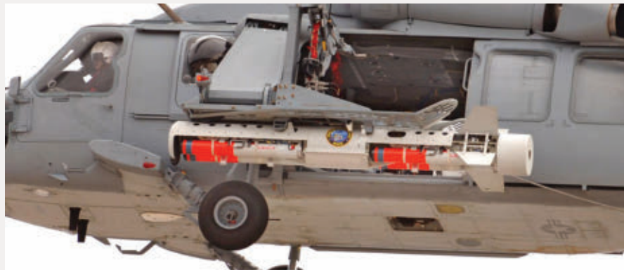
The Raytheon Airborne Mine Neutralization System uses a mine-destroying unmanned underwater vehicle (UUV) that takes its control from the helicopter's common console.
